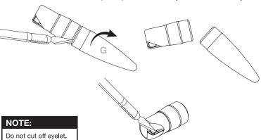
If needed, add tape to base of both nose cone pieces and insert pieces into both ends of clear payload tube H.
