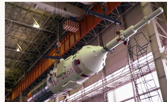
The escape tower, Soyuz spacecraft, and second stage are ready for integration with the lower portion of the TMA-8 booster vehicle. (NASA)
