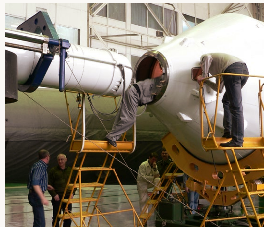
Vital for crew safety, the escape tower mast is attached to the aerodynamic spacecraft fairing of Soyuz TMA-8. (NASA)
