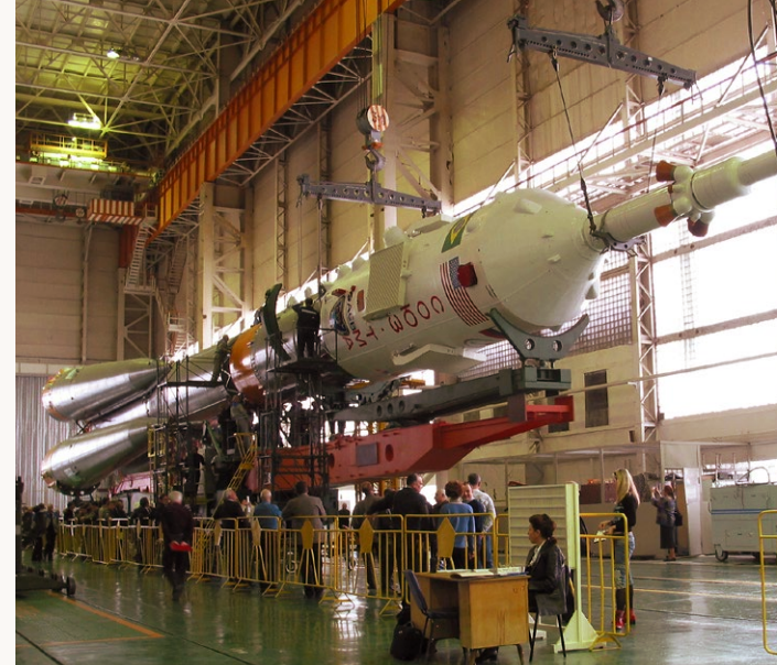
The integrated escape tower, spacecraft faring, and second stage of Soyuz TMA-8 are carefully positioned for mating with the lower portion of the booster at the Baikonur Cosmodrome. (NASA)
