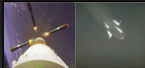
The spent side boosters fall away from the central core of the Soyuz booster in a distinctive pattern called the “Korolev Cross.” (ESA)
