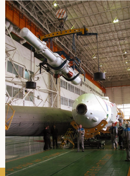
In the vehicle integration hall at the Baikonur Cosmodrome a crane moves the escape tower into place for mounting onto the spacecraft fairing. (NASA)
