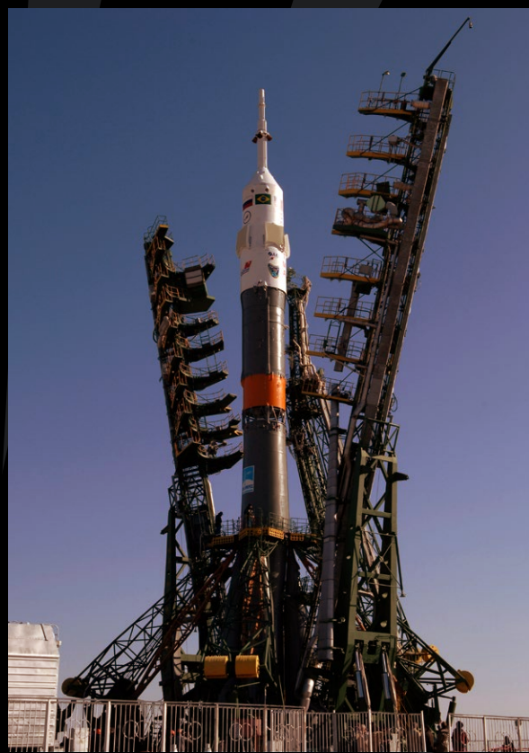
Left: When the Soyuz rocket is in place on the launch pad, service arms close around the rocket, allowing access for service, fueling, and crew access. The arms retract in the final stage of the countdown. (NASA)
