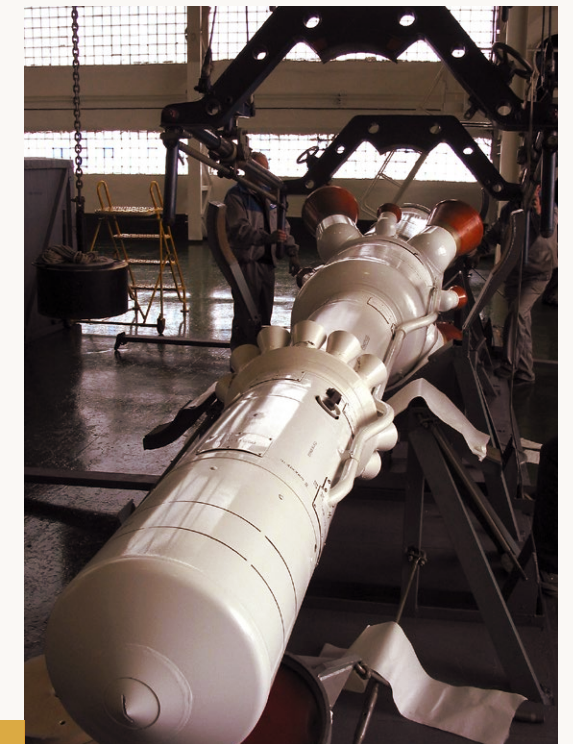
The escape tower is prepared for installation atop the Soyuz TMA-8 spacecraft. (NASA)
