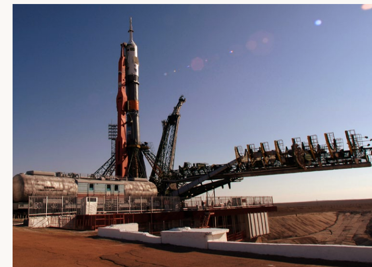
Once the Soyuz booster and spacecraft have been fully integrated it is slowly moved from the assembly hall to the launch pad by rail. The special rail car on which the rocket is mounted is designed to provide power, cooling, and fluid support to the booster during the short journey. (NASA)
