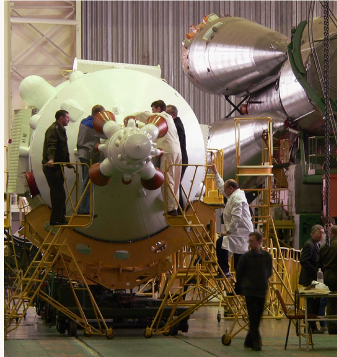
In the integration hall at the Baikonur Cosmodrome technicians inspect the separation plane between the escape tower and the spacecraft fairing.
