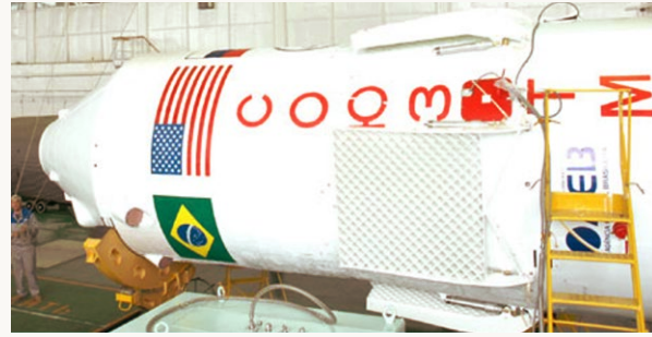
In the event that the escape tower is activated, the grid fins on the sides of the spacecraft fairing will quickly swing down into position, providing passive stability during boost. (NASA)
