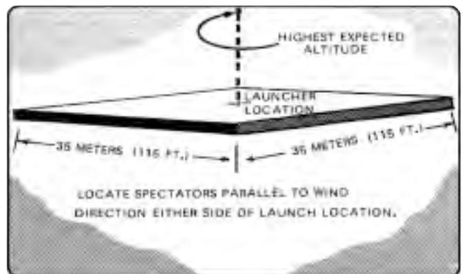
The launch site for the contest should be at least 35 meters (115 feet) on a side. The launch area's smallest dimension should be no less than one-fourth of the highest anticipated altitude. No launches should take place from less than 10 meters (33 feet) from any edge of the area being used.
