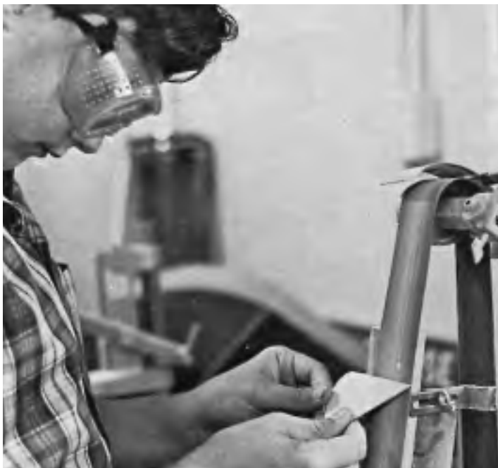
Advanced rocketeer airfoils special competition designed fin on workshop sander.
