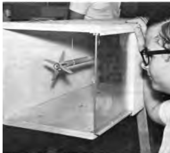
Rocketeer tests the stability of his model rocket in the club wind tunnel.
