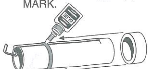
E. SLIDE GREEN ADAPTER RING ONTO ENGINE MOUNT TUBE DOWN TO THE 3/4" (19 mm) MARK.
