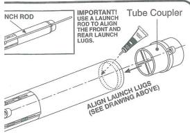
B. Apply a ring of just inside the upper end of the Medium Red Bubble Body Tube and slide the Tube Coupler into the tube. Before glue sets, align the Launch Lug on the Coupler with the Launch Lug on the Engine Mount.
